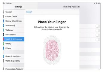
Place your finger on the touch sensor (Home button). You're asked (via an on-screen message) to lift your finger and then place it back on the Home button, until all the grey fingerprint lines are red.
